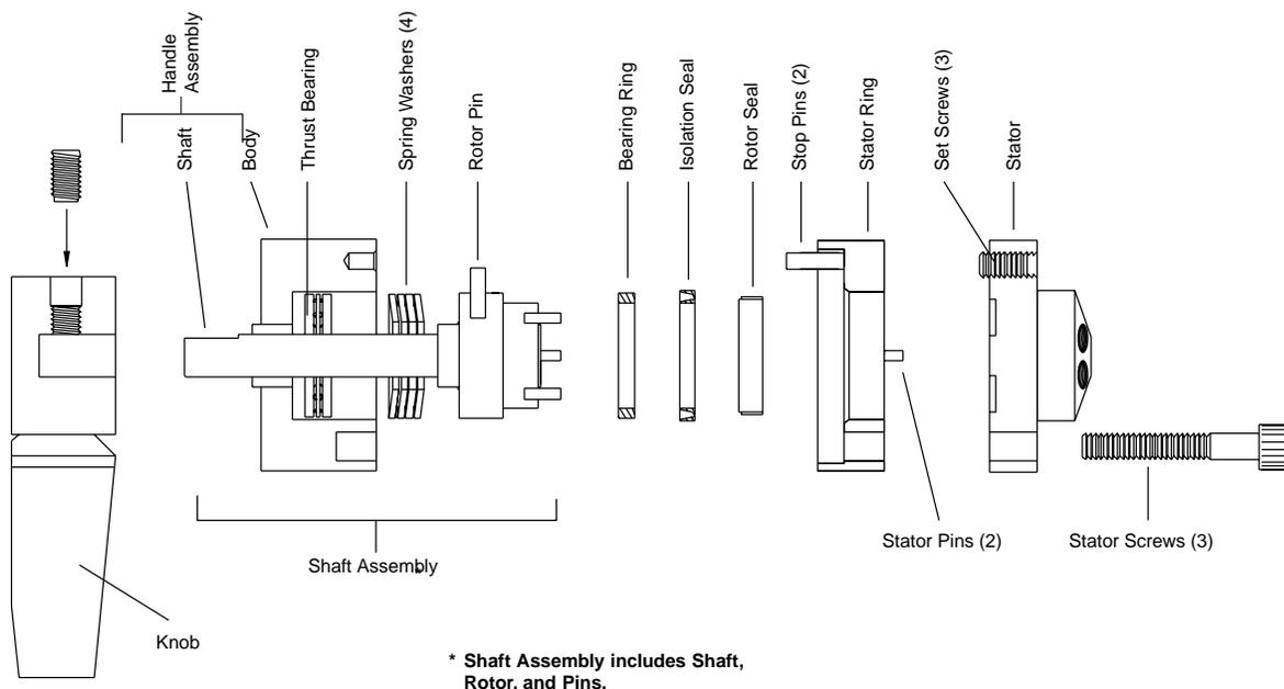
Fig. 4. Exploded view of Type 70 valves.
