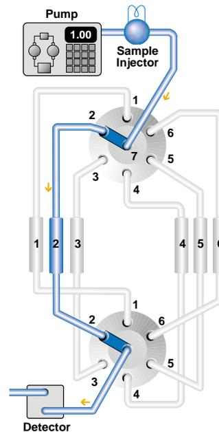
**Fig. 10. Six column selection using two Model 7060 switching valves.**
