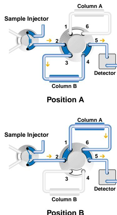
**Fig. 7. Two column selection using Model 7000.**
