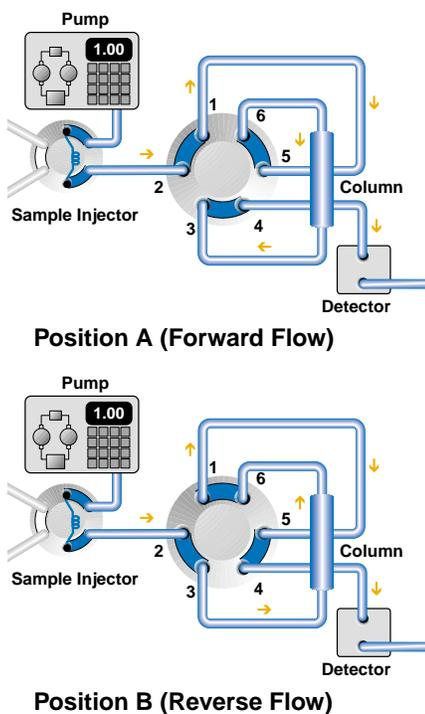
**Fig. 8. Illustration of column flow reversal for backflushing using Model 7040.**
