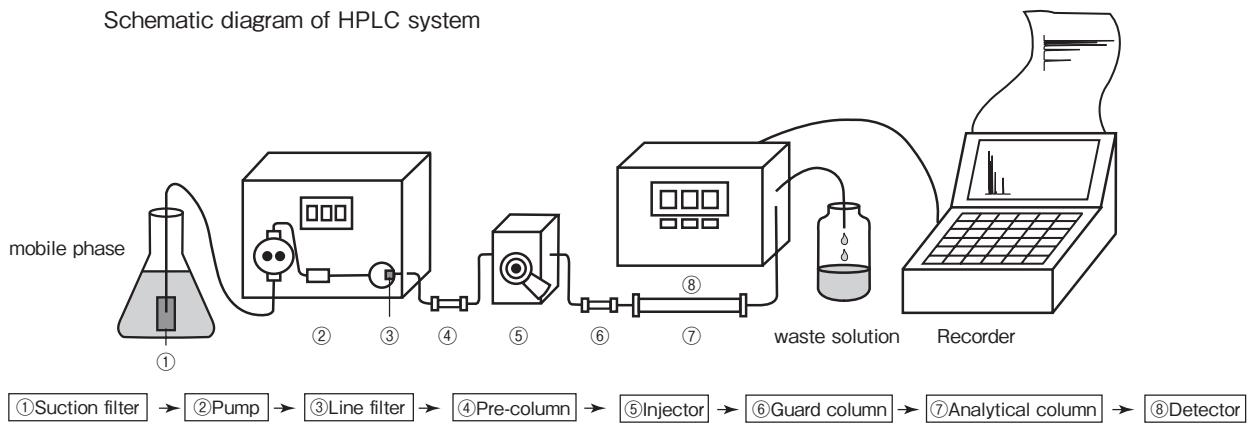
①Suction filter → ②Pump → ③Line filter → ④Pre-column → ⑤Injector → ⑥Guard column → ⑦Analytical column → ⑧Detector
