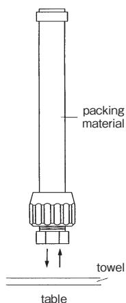
1. Wash the column in methanol and mount the end fitting on the bottom of the dried glass column as shown in the diagram to the left.
