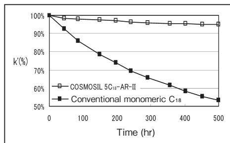
Figure. Decomposition test in 0.1% Trifluoroacetic Acid solution at 60°C.
