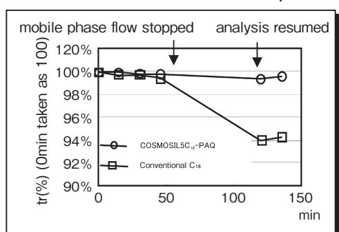
The figure shows the change of retention time for thymine with 100% aqueous mobile phase (20 mmol/l phosphate buffer pH7). The sample was analyzed 4 times. Flow of mobile phase was then stopped for 1 hour. The sample was analyzed under the same condition again after 1 hour. The conventional C<sub>18</sub> column showed change of retention time, but COSMOSIL 5C<sub>18</sub>-PAQ maintained stable retention time.
