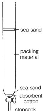
1. Use a standard open glass column, close the stopcock, pack a small amount of absorbent cotton in the bottom of the column and add solvent to approximately 1/3 of the column length.
