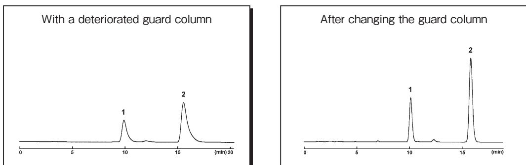
Column            COSMOSIL 5C<sub>18</sub>-MS-II 4.6 mm I.D. × 150 mm
