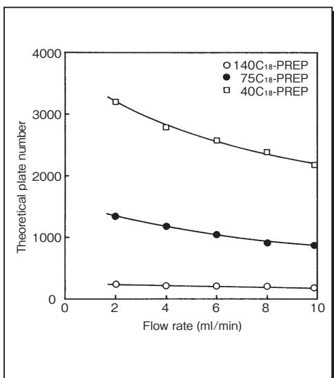
Figure 2. Flow rate against theoretical plate number
